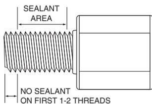
**Note:** If Teflon tape is used, it should be wrapped no more than 1 1/2 to 2 turns in a clockwise direction when viewed from the thread end.
